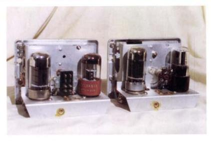
Fig. 2: Before conversion (left) and after re-building (right) the 'PB' transmitter is re-born from the audio amplifier unit (see text).
