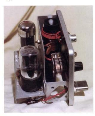
got one of the PB units) you'll find there are five chassis mounted decoupling capacitors, these make ideal mounting points for the h.t. rail and all the components that emanate from it.
